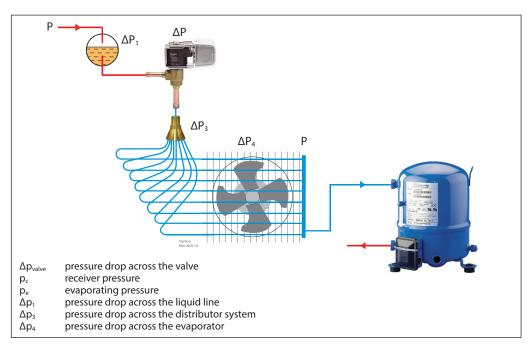
Note! The pressure drop across the liquid line and the distributor system must be calculated on the basis of the valve's max. capacity, as the valve operates with pulse-width modulation.
