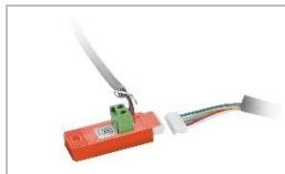
The device supports different baudrates (par. **bAU**) and parity control (par. **PAr**). Please check the serial network to adapt them according to the other devices. The **XJ485CX** serial interface is required to convert the TTL output into an RS485 signal.
