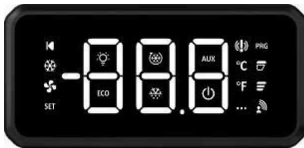
XR70T has a capacitive user interface with Full Touch technology. The whole display area is used to interact with the device. Specific gestures are used to enable or disable functions, browse through screens and operational modes and modify the configuration of the device.
