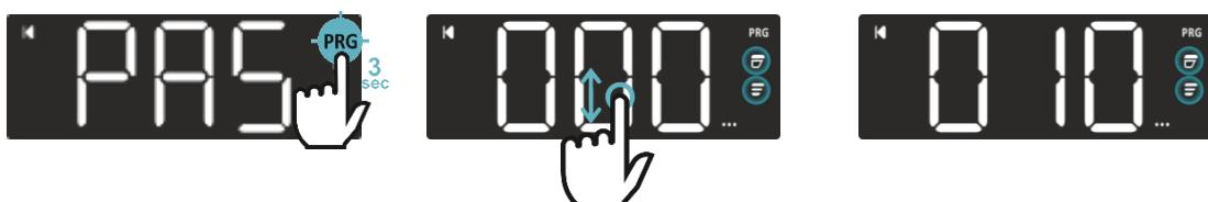
When in the **PAS** group, it is possible to set the password value by touching the **PRG** icon for 3 sec. V-swipe on a single digit to modify the value, then confirm the password value by touching the **PRG** icon for 3 sec.
